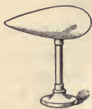
FIG. 282.—Electrical Density is Greatest at the Pointed End of this Conductor.
